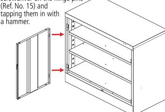
**11.** Attach the right door (Ref. No. 9) to the unit in the same way you attached the left door.
