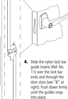
**5.** Attach the "dummy" handle (Ref. No. 13) using two #8-32 X 1/4 hex-head bolts and lock washers.
