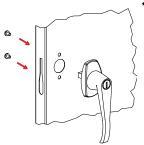
**1.** Place the locking handle (Ref. No. 9) on the right hand door and fasten with two #8-32 X <sup>1</sup>/4 hex-head bolts and lock washers, provided with the handle.
