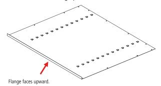
**3.** Attach the left side (Ref. No. 2) to the back by placing flange (A) around the back and bolting the back and side together with four bolts and nuts (Ref. Nos. 17 & 18). Be sure that the lances on all shelf adjustment strips (B) point in the same direction.
