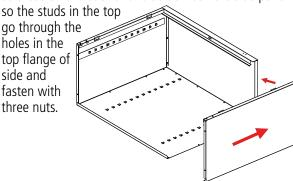
**6.** Attach the sill (Ref. No. 5) to the sides. Place nuts loosely on each of the studs and slide the ends of the sill into the slots on both sides of the unit. Then, securely tighten the nuts.
