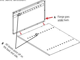
**4.** Attach the top (Ref. No. 7) to the unit by sliding the outer flange over the back of the unit and the side flange to the side panel on the unit. The threaded studs should go
