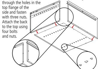
**5.** Attach the right side (Ref. No. 3) to the back in the same manner as you did in step 3, again making sure that the flange is around the back and that the lances on the shelf adjustment strips are pointed in the same direction as those on the back and left side. Push the side panel up so the stude in the top.
